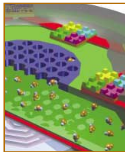
A nanopore membrane protects insulin-secreting cells from anti-bodies.
